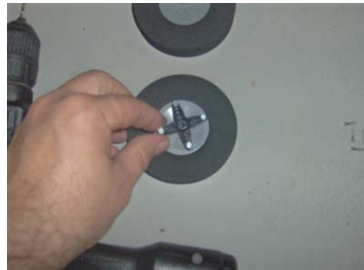
Step 11: Drill 4 small holes (1/16”) for servo horn. Use the servo horn as a template; this makes it much easier to thread the screw. If you don’t have a 1/16” drill bit the screws can be driven manually.
