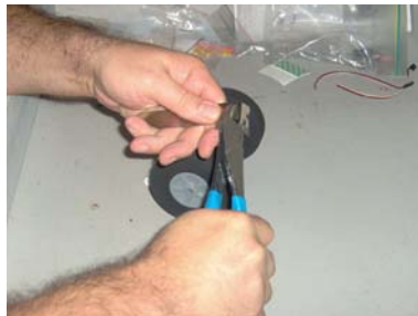
Step 13: Cut the right-angle top from the PC-slot cover. You will have to use a pair of “dikes” (diagonal cutters); you may have to bend it back and forth to break it.
