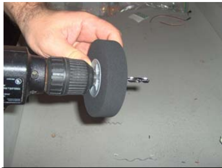
Step 10: Prepare the wheels: Drill out center bore to 1/4”. If you don’t do this the servo screw will not fit!
