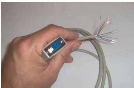
Figure 5: Strip the individual wires on the cut end.
