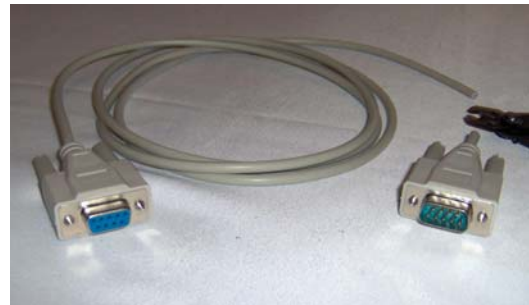
Figure 3: cut off the end opposite the DB9 pin female connector. If you’re using a modem cable the cut end will be a DB25.
