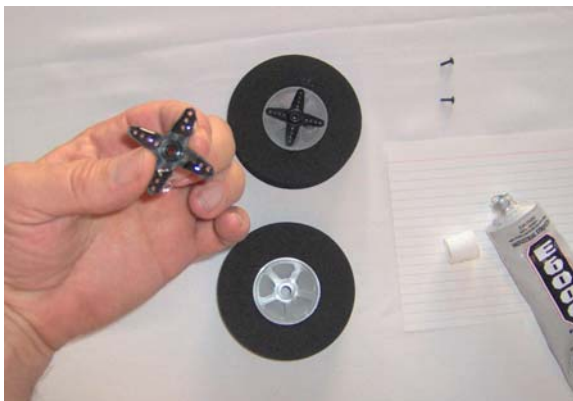
Figure 22: Put a dab of E6000 on each leg of the servo horn. Be sure and apply glue to the side opposite the cap into which the servo plugs.
