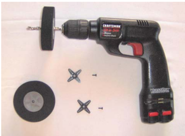
Figure 21: Before gluing the servo horn to the wheel drill out the wheel to 1/4" so the servo screw can pass through. Do this before gluing the servo horn to the wheel!
