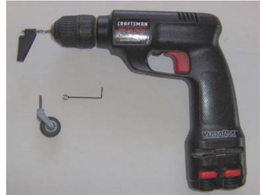
Figure 16: Drill out the bracket shaft to 9/64" so to accommodate the 1/8" Klett Plastics fork shaft. Drill it out before gluing!
