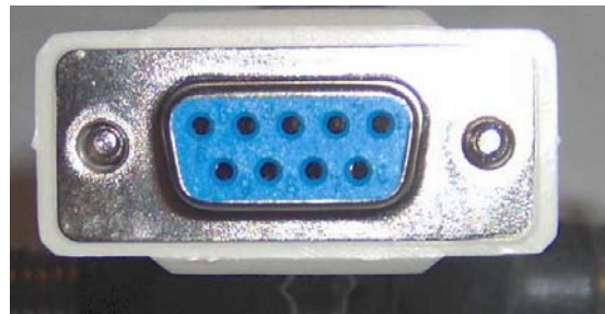
Figure 7: If you look closely at your female DB9 connector you can read the numbers. You may need a light and/or magnifying glass.
