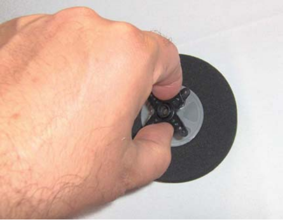
Figure 23: Place the horn on the wheel (cap facing up). You can center it by aligning the four spokes with the outer rim of the hub. Let it sit overnight to cure.
